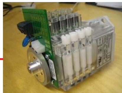
Encoder in the end of rotating limit switch (Stromag)
